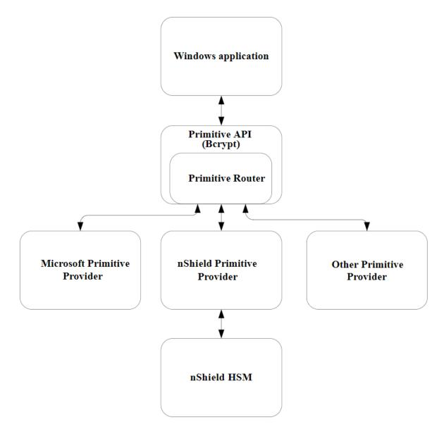
For an illustration of communication between the architecture layers for cryptographic key storage, see the following diagram.
