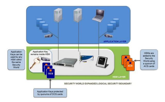
The Security World technology makes sure that keys remain secure throughout their life cycle. Every key in the Security World is always protected by another key, even during recovery and replacement operations. Because the Security World is built around nShield key-management modules, keys are only ever available in plain text on secure hardware.
