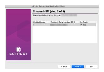
In the example screen shown, an HSM will not be **Remote Administration (RA) Ready** until it has the appropriate firmware, and has one or more dynamic Slots configured.
