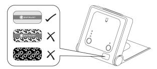
• Where possible, use the lock slot of the nShield Edge to secure it to a desk with a compatible lock (not supplied).
