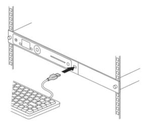
Instead of using the controls on the front panel to configure the nShield 5c, you can use a US or UK keyboard. You might find a keyboard easier for entering dates and IP addresses. You connect the keyboard to the USB connector on the front of the nShield 5c.
