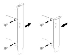
To fit the full height bracket to the module:
