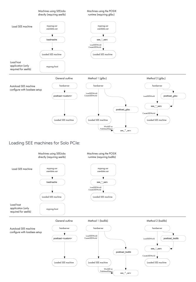
You can load SEE machines manually by running the **loadmache** command-line utility or, optionally, you can load SEE machines that require support from a host-side see-\*-serv util ity by specifying the -M option when you run the utility.
