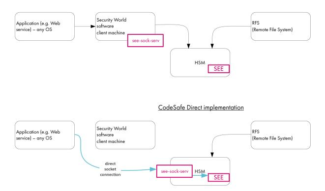
The nShield Connect can be configured to receive direct socket connections from the SEE machine via see-sock-serv, removing the need for a client machine. You do this by specifying postload\_prog and postload\_args in the load\_seemachine section of the nShield Connect hardserver configuration file, located in NFAST\_KMDATA/hsm-<ESN>, where <ESN> is the Electronic Serial Number of the HSM. (For more information about this section of the configuration file, see load\_seemachine.
