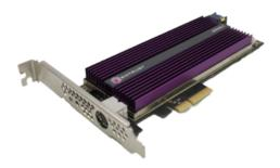
The nShield 5s is a new HSM based on the PCIe form factor. The hardware is similar to that of the nShield Solo XC with the following main differences:
