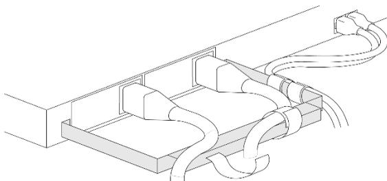
5. Ensure that the cable connectors are still firmly inserted.
