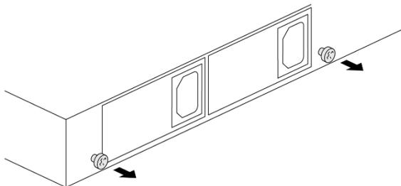
2. Fit the cable retainer by hooking it on the loosened screws, and then tighten the screws.
