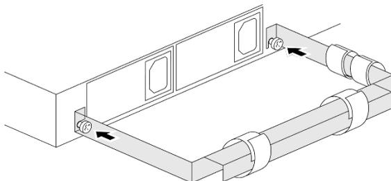
3. Connect the power cables and network cables to the nShield Connect, as described in the *nShield Connect Installation Guide*.
