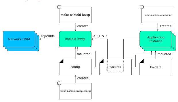
The nshield-hwsp container runs the hardserver. It is supplied with configuration to connect to one or more network HSMs (nShield Connects). It exposes the hardserver via an AF\_UNIX socket.
