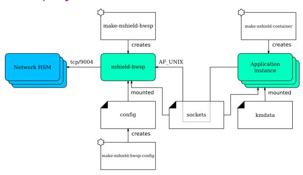
The nshield-hwsp container runs the hardserver. It is supplied with configuration to connect to one or more network HSMs (nShield Connects). It exposes the hardserver via an AF\_UNIX socket. Access to the hardserver socket must be restricted to trusted users.
