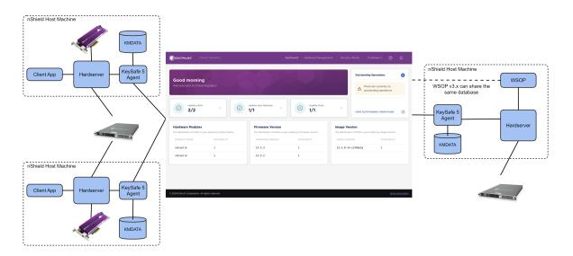
KeySafe 5 can be deployed as a Kubernetes application to manage a large estate of HSMs, or ran in single binary executable format to manage a single nShield Security World host machine and attached HSMs, see KeySafe 5 Local.
