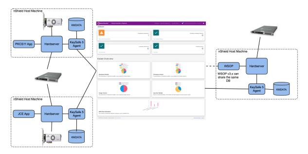
The main central management platform of Keysafe 5 is deployed as either a Kubernetes application or as a cluster of Virtual Machines (VMs). For each nShield client machine that you want to manage using this platform, you must install a Keysafe 5 agent binary alongside the existing nShield hardserver.
