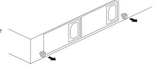
Fit the cable retainer by hooking it on the loosened screws, and then tighten the screws.
