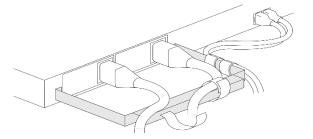
5. Ensure that the cable connectors are still firmly inserted.
